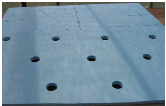
Figure 10. An electric drill with a 2-inch hole saw is used to cut holes in the top cover sheets at the layout marks. A template with a suggested plant spacing on a 2 x 4-ft tank cover sheet with a density of 1.5 plants per square foot is shown.
