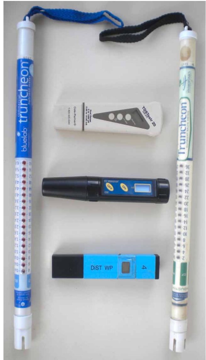
Figure 12. Different models of electrical conductivity (EC) meters to measure total fertilizer salts in milli-siemens (mS).
