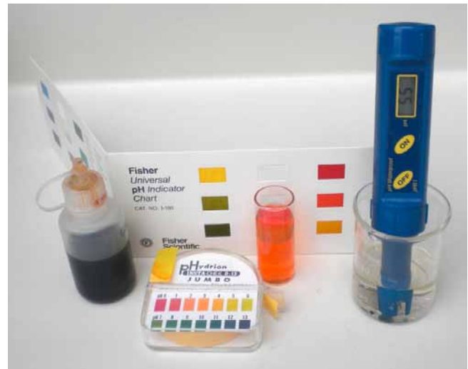
Figure 14. Alternatives for measuring solution pH are a pH meter, a pH test kit, and pH indicator paper.
